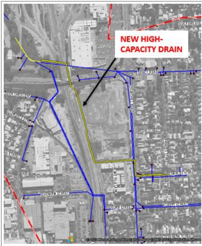
Figure 1: Stage 1 of Churchill Road Drainage Upgrade – HEP Channel to Charles Street
